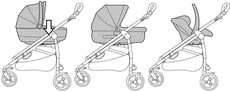
23 Surefix is a fast and practical system that allows you to attach the car seat or the carry cot to the Surefix Base of the chassis in one quick step. Place the item on the Surefix Base and press down with both hands until it clicks into place. Always apply the chassis or stroller brake before attaching and removing products (refer to the respective instruction manuals). Check that the child transport unit is properly attached.
